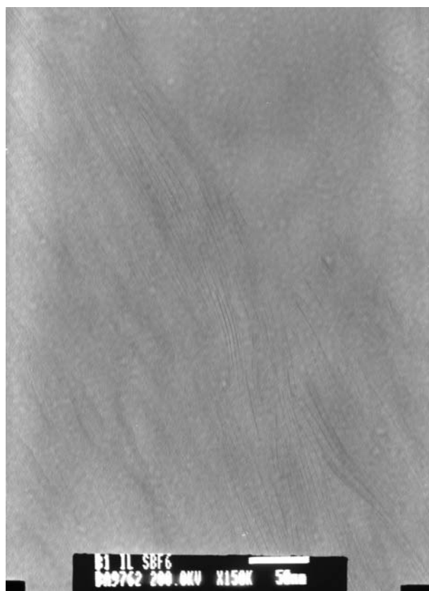
Figure 12 Transmission electron micrograph of epoxy nano-composite with 5 wt.% Nanomer I30E.
