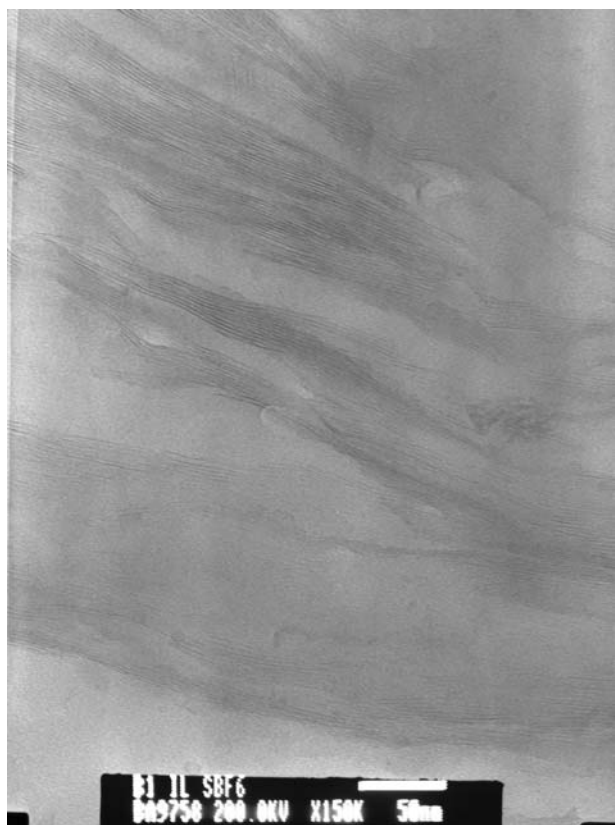
Figure 11 Transmission electron micrograph of epoxy nano-composite with 5 wt.% Cloisite 25A.
